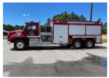
Updated pictures of the tanker (previous newsletter had the chassis) The Pumper/ Tanker has been in service, this apparatus holds 3300 gallons of water and has a 2000 gallon per minute pump.
